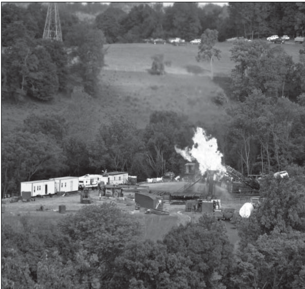
Figure 4.5. In June 2010, a drilling operation on a gas well in Marshall County, West Virginia, struck an abandoned coal mine triggering a blowout and explosion that injured seven workers (three seriously).
