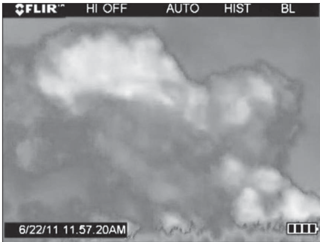
Figure 6.1. A cloud of methane gas emitted into the atmosphere as a result of venting during the completion of a natural gas well in Susquehanna County, Pennsylvania, June 22, 2011. This image is from an enhanced infrared photograph.
