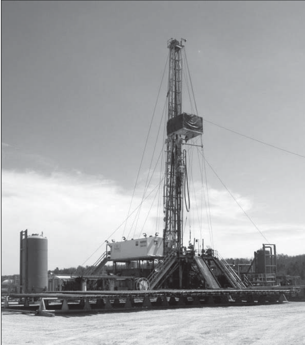
Figure 3.1. A Marcellus Shale drilling rig outside Towanda, Pennsylvania. A drilling rig stays on site for only the duration of the drilling of the well or wells, and can be assembled or disassembled in the course of a few days. The drilling operation itself lasts several weeks for each well; several wells could be drilled on the same well pad, so the duration that a drilling rig stays on site can vary.
